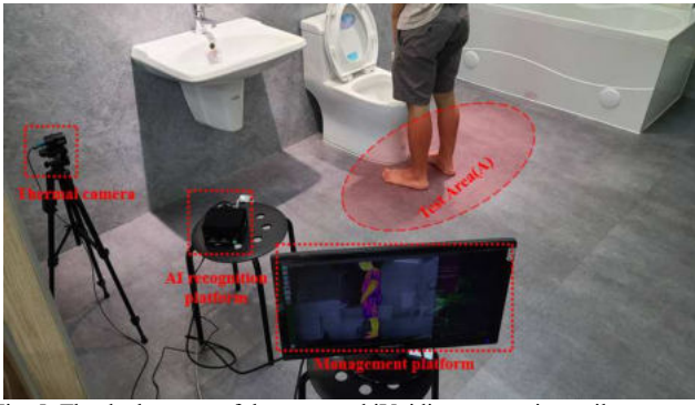
Fig. 5. The deployment of the proposed iVoiding system in a toilet.
