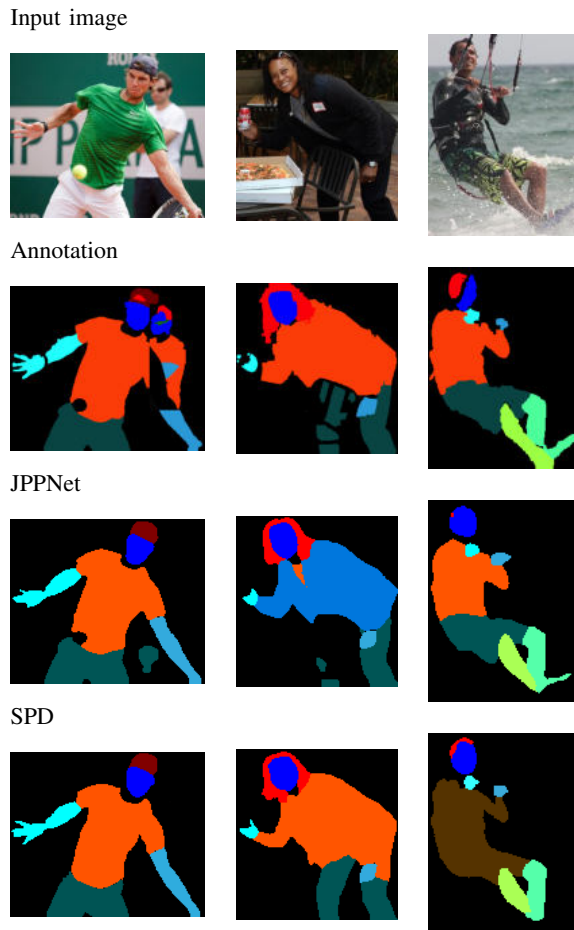
Fig. 7. Comparison of the segmentation results generated by the proposed SPD model and the competing JPPNet on selected images from the LIP dataset. The first row showed the selected input images, the second row shows the ground truth annotations, whereas the third and fourth row show results for JPPNet and SPD, respectively.
