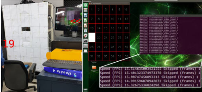
Fig. 11. Our experiment with the optimal camera position at 55.5 cm from the top of the shelf. A user gazes at rectangle number 19 (leftmost side). Our gaze estimation module correctly identifies the user's gazing (shown in a white rectangle). It skips one to five frames in order to process real-time images captured from the camera. The processing speed is about 10 to 15 FPS.
