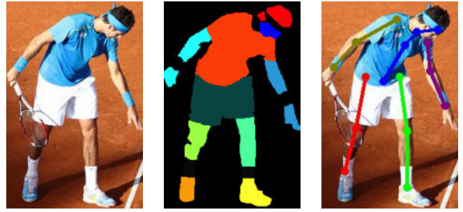
Fig. 6. Example image from the LIP dataset and the corresponding segmentation masks and 16-point skeleton markup.
