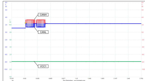
Fig. 16. CAN internal Loop-Back Mode with invalid WUF
