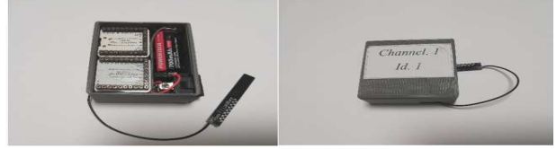
Figures. 2. a. the combinations of Microduino boards with 3.7VDC battery, b. final WSD inside 3D printed box.
