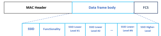
Fig.5 packet frame design for notification messages coming from the UAV to the Ground (Routers and Gateways)
