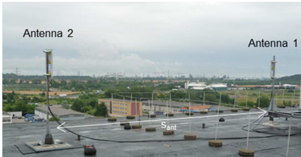
Figure 2.1: eNB antenna configuration and view to the motorway. The antenna separation s_{ant} is varied between 0.2 m and 15 m.
