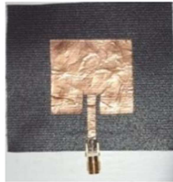
Fig 9. Fabrication of conventional antenna front view.
