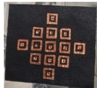
Fig 11. Fabrication of EBG antenna front view.
