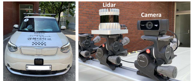
Fig. 1. Sensor configuration for the multimodal object detection and ranging.
