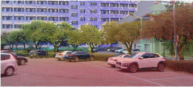
Fig. 2. Projection of the 3D lidar points on the 2D camera image.
