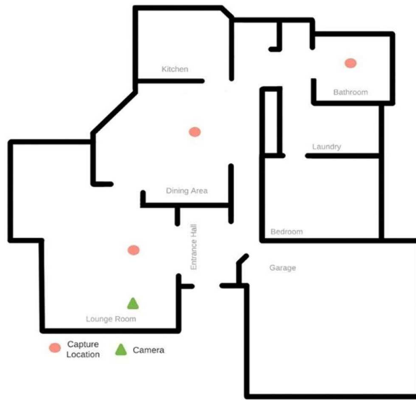
Fig. 4. Camera placement and Wi-Fi signal capture locations in 45-degree increment
