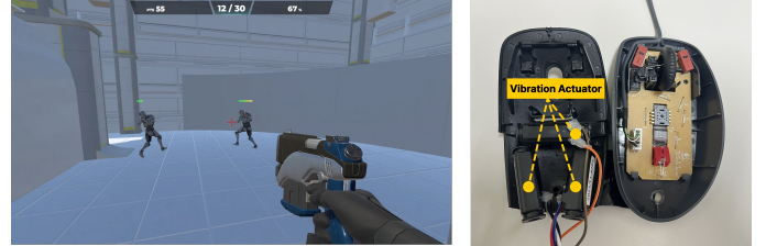
Fig. 1. (Left) Game interface used in the experiment. (Right) A custom haptic mouse equipped with three haptic actuators.
