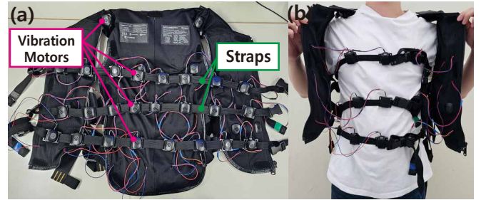
Fig. 2. The customized haptic suit (a) and its worn appearance (b).
