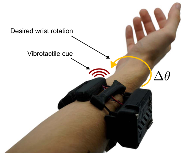
Fig. 1. Vibrotactile wrist rotation guidance. The wearable haptic device applies vibrotactile cues to communicate the desired wrist rotation \Delta\theta to the human user.
