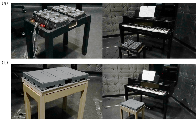
Fig. 3. A haptic feedback device (a) and a sensor device (b) designed to replicate the conventional shape of a piano chair.
