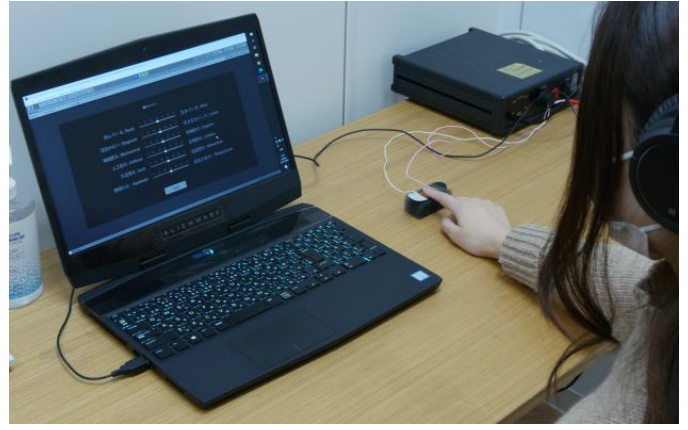
Fig. 1. Experimental setup for Experiment I (Animacy Test). Participants received haptic stimulation patterns through the pad of their right index finger using the haptic display, and evaluated the perceived animacy of each stimulus using the questionnaire displayed on a PC screen in front of them.
