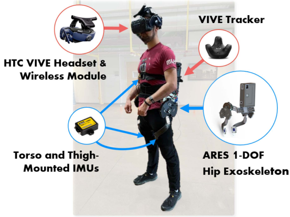
Fig. 9. The sensors and wearable devices worn by subjects during the experiment.
