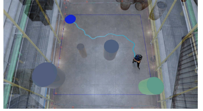
Fig. 8. A visualization of the virtual reality environment overlapped with the physical experimentation space. The subject's path is outlined in light blue. The obstacles are shown in gray. The start and goal are the blue circle and green cylinder, respectively.
