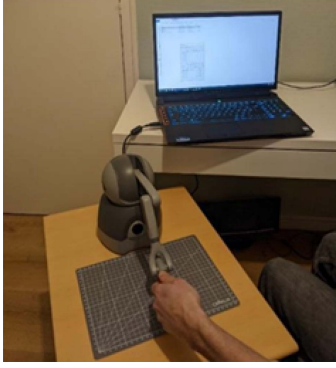
Fig. 12. Kinesthetic evaluation platform with the geomagic touch stylus held with the non-dominant hand.
