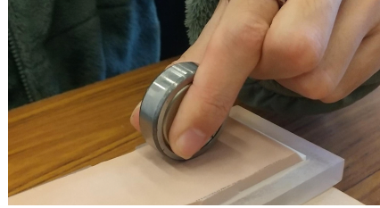
Fig. 1: Shaft ball bearing and grabbing methods. (a) Shaft ball bearing used in the experiment as a medium for participants to interact with the artificial skin. (b) Only the inner ring was held by fingers in the rolling condition. (c) Both the inner and outer rings were held by fingers in the sliding and pressing condition.
