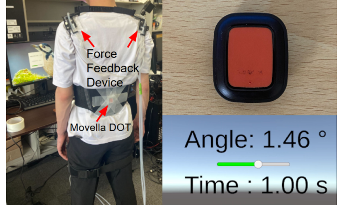
Fig. 3. Experimental setup. Left: Experimental scene with the force feedback device on the shoulders and the IMU sensor on a waist belt. Top right: The Movella DOT IMU sensor. Bottom right: Real-time tilt angle display for participants.
