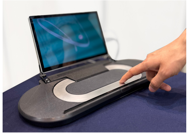
Fig. 1. The flatLoop device provides rich tactile feedback using active force across various user interfaces.
